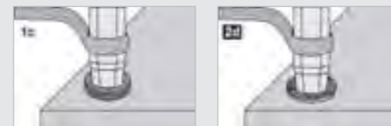
Slide in the box spanner to the bottom and screw out without tilting
