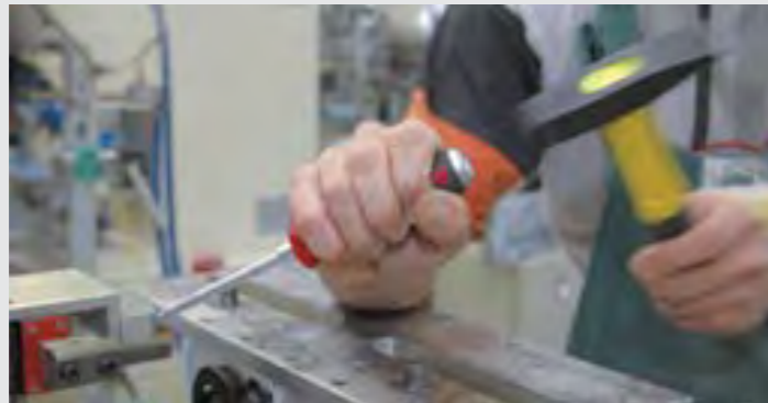
The solid steel cap at the end of the SoftFinish® handle enables controlled hammer blows, for example, when loosening a tight screw.
