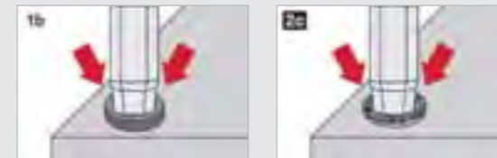
Firmly hammer in the screw extractor with a hammer
