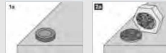
Damaged or rounded allen screws or... ... broken off screw heads
