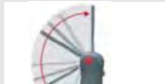
The 180° stop limit when working on applications with higher safety requirements puts an end to trapped fingers.
