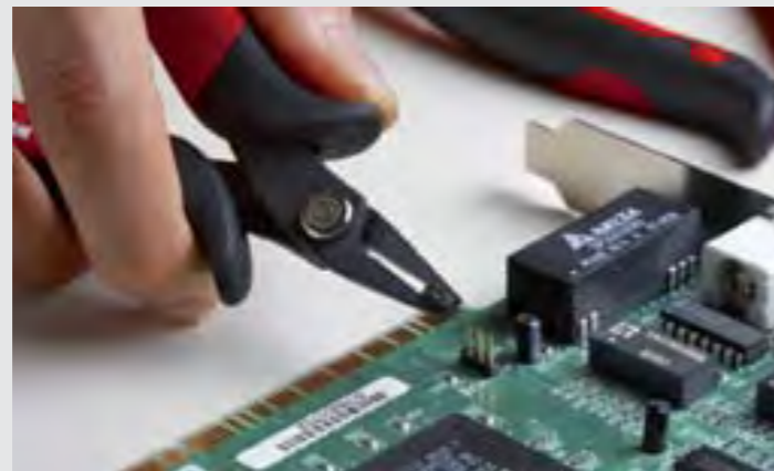
The Electronic long-nose pliers from Wiha hold small components and bend wires.
